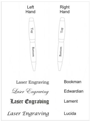
It is always better to engrave before assembly of the pen so the clip doesn't impede the engraving because of the slight curve involved.
